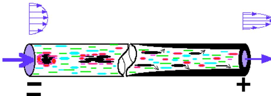
*Figure 12: Deposition and plugging of petroleum flow conduits due to streaming potential generated and sticking of asphaltene particles to the walls.*
