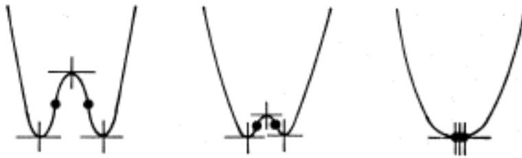
Figure 17. Variation of the free energy graph in the case of a 2 → 1 phase transition at a bicritical point. (From Ref. 110.)
