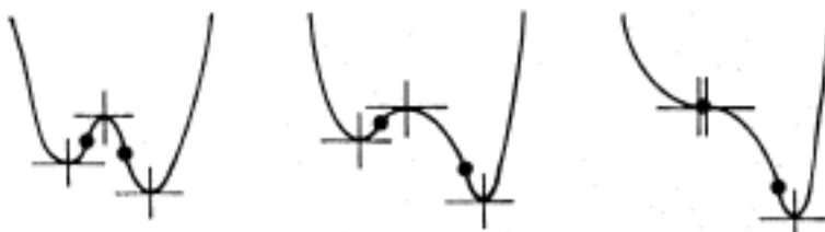
Figure 18. Variation of the free energy graph in the case of a 2 → 1 phase transition at a monocritical point. (From Ref. 110.)
